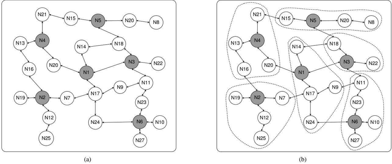
Fig. 2. An example of 2-hop clusters: (a) before handshake, and (b) after handshake
